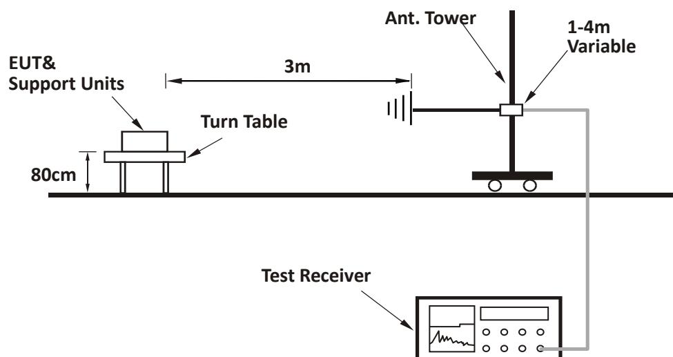
**TEST REPORT****For Radiated emission above 1GHz:**
