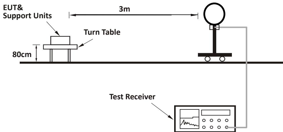
**For Radiated emission 30MHz to 1GHz:**
