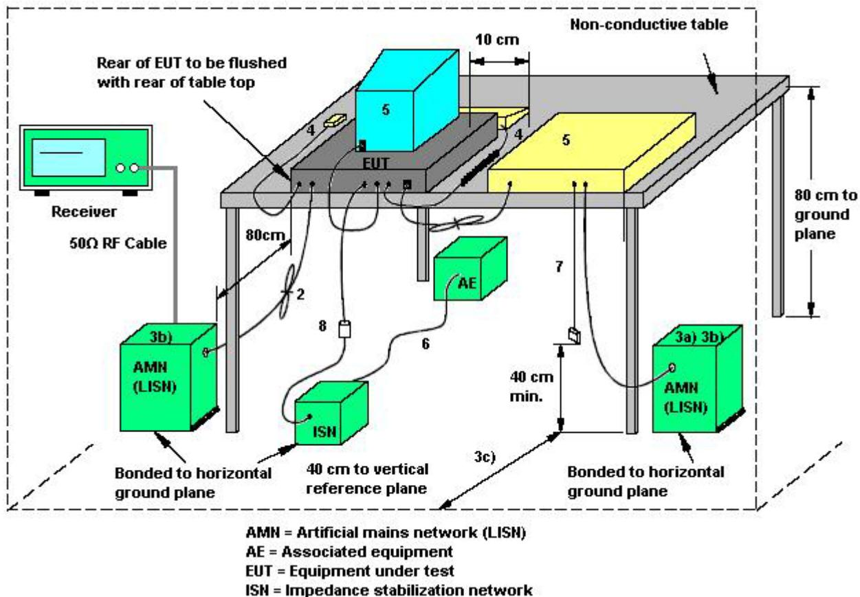
1. If cables, which hang closer than 40 cm to the horizontal metal groundplane, cannot be shortened to appropriate length, the excess shall be folded back and forth forming a bundle 30 cm to 40 cm long.
