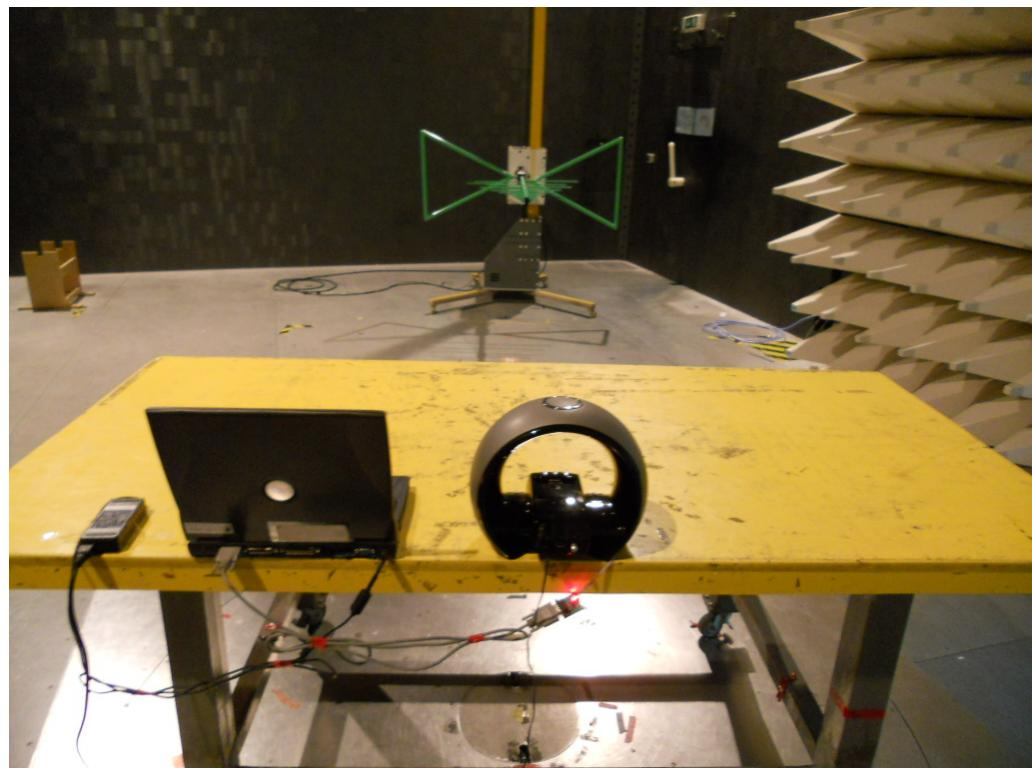
**For radiated emissions above 1GHz****FRONT VIEW**
