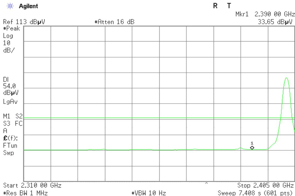
**Detector mode: Peak****Polarity: Horizontal**
