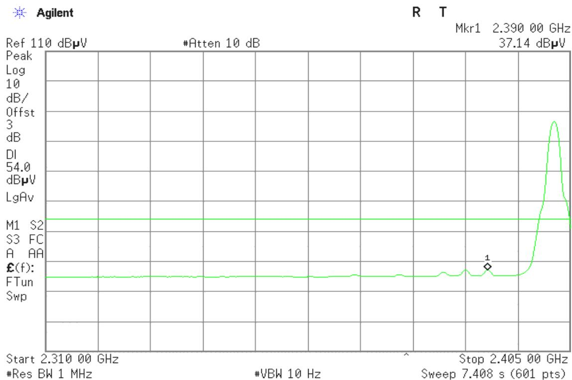
**Band Edges (CH High)****Detector mode: Peak****Polarity: Vertical**
