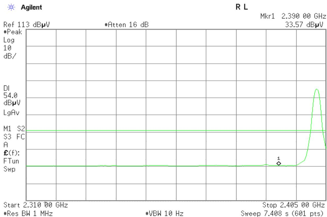
**Band Edges (CH High)****Detector mode: Peak****Polarity: Vertical**
