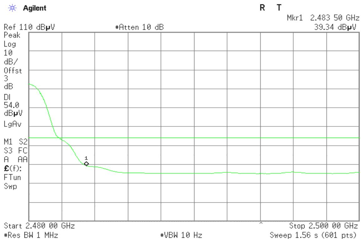
**For 8DPSK / DH5****Band Edges (CH Low)****Detector mode: Peak****Polarity: Vertical**
