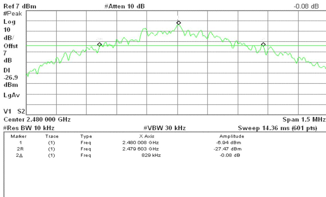
**For 8DPSK / DH5****20dB Bandwidth (CH Low)**
