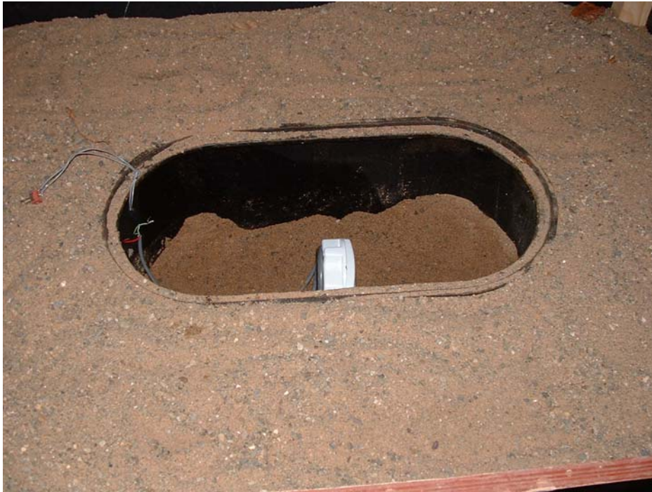
PHOTOGRAPH No. 2 TRANSMITTER TOP VIEW WITHIN THE ' PIT '
