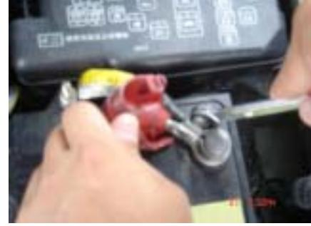
5. Connect vehicle Pos.(+) cable to the Post Adapter of I.B./ R.I.B.
