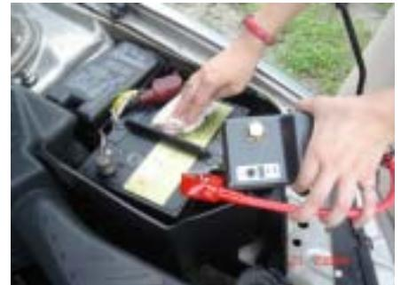
3. Use the double sided 3M foam tapes to stick the back side of I.B./R.I.B. for attaching on the battery.
