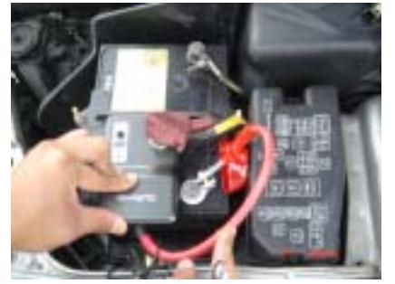
7. Release Neg.(-) battery cable from Neg.(-) battery post, then install the black ground wire with the U-clip securely to assembly.
