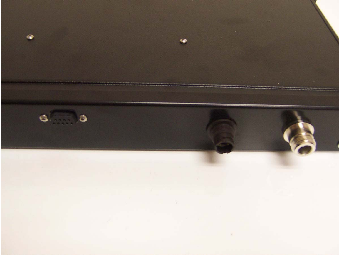
Close-up of external connections of the RC 2500 collector
