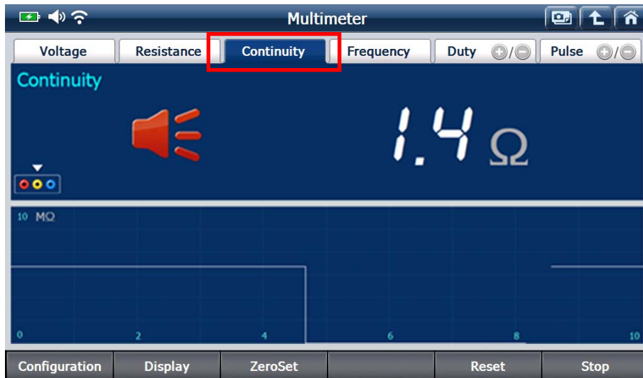
[ Continuity Test – Normal / Buzzer Sounds ]
