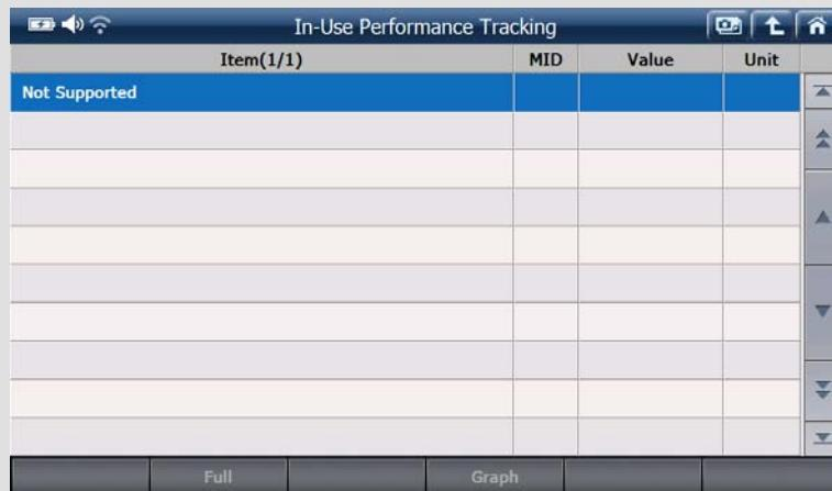
In order to view the Current Data in graphical form, select the “Graph” button in the bottom. And the “Text” button will switch to the numeric mode again.
