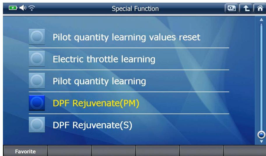
Find and select the desired special function from the list, read the instruction provided on the screen carefully and select “Start” or press the [F1] key to start.
