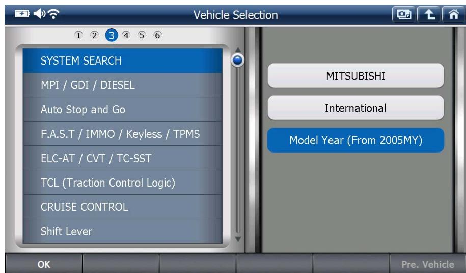
If International is selected, a simple Diagnostic Connector Type selection follows and then the system selection can be made without having to follow further model name, model code, type or model year selections.
