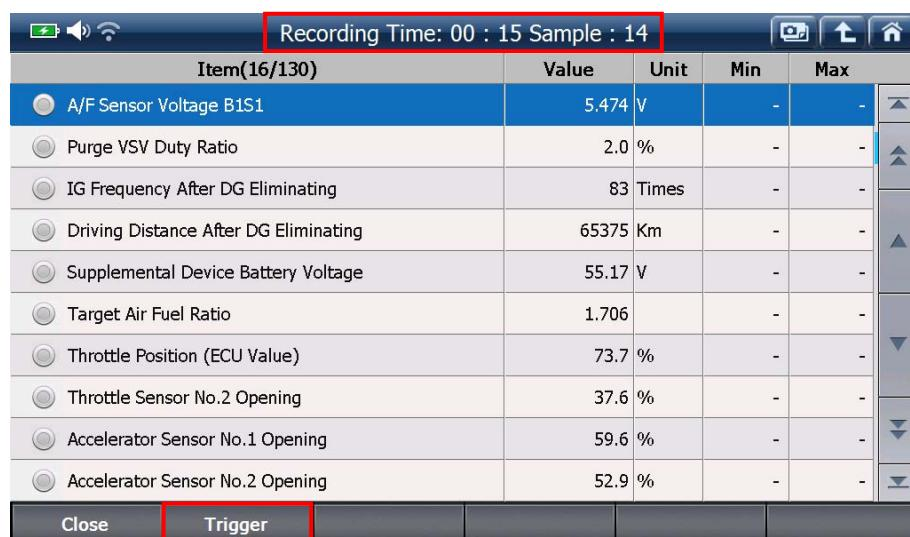
Select “Trigger” to mark the important or critical moment, which is going to be indicated when reviewing the data.
