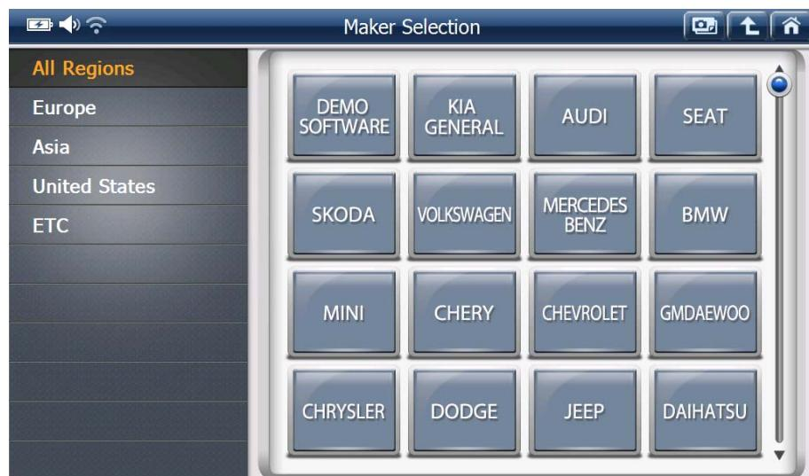
The brand of the vehicle that the G-scan2 has recently communicated with is placed in the top of the list. By applying this so called “Recent-First” rule, the more frequently serviced vehicle brands are placed in the first 1 or 2 pages of the list, and the rarely used brands are listed in the bottom of the list.
