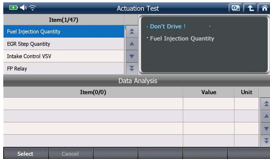
Control On/Off or adjust the values up and down using the buttons and keys and check the response of the selected active parts and the vehicle control system's reactions by monitoring the live data provided in the lower half of the screen.
