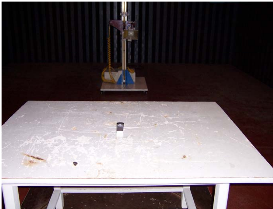
Field Strength Emissions Test Set-up (Above 1GHz)
