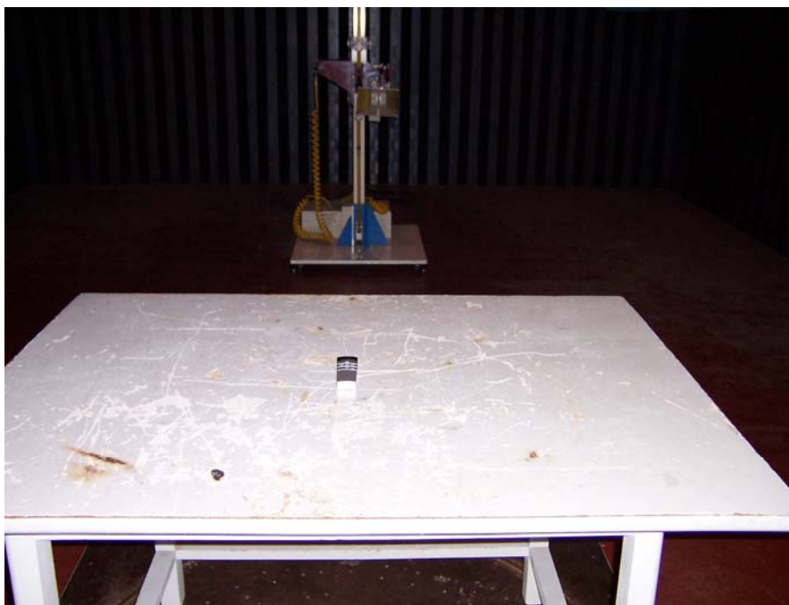
Radiated Emissions Test Set-up (Above 1GHz)
