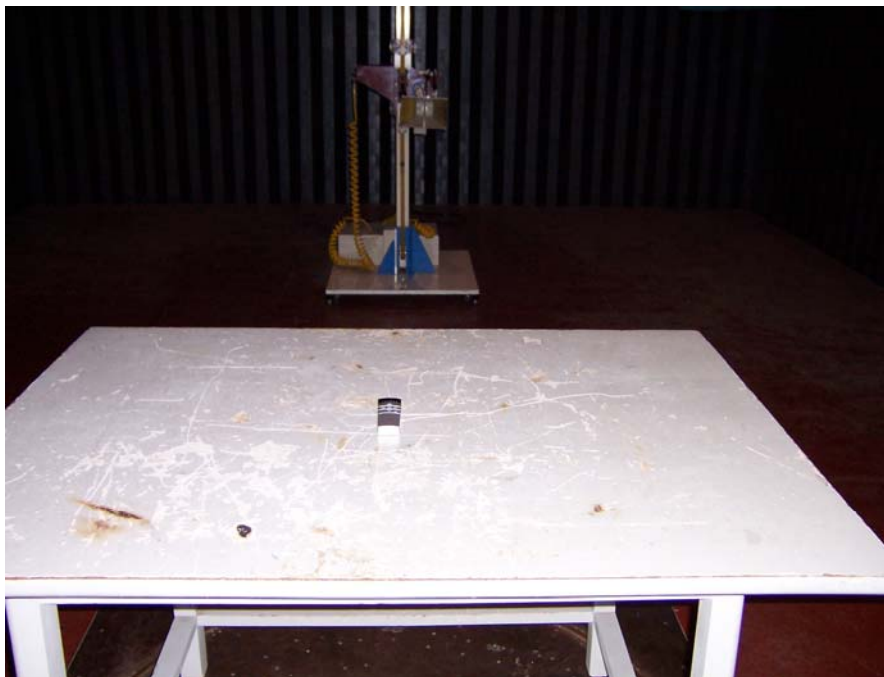
Field Strength Emissions Test Set-up (Above 1GHz)
