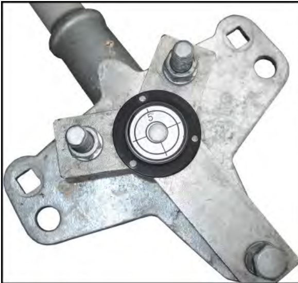
Figure 35: Magnetic level on adjustable leveling bracket
