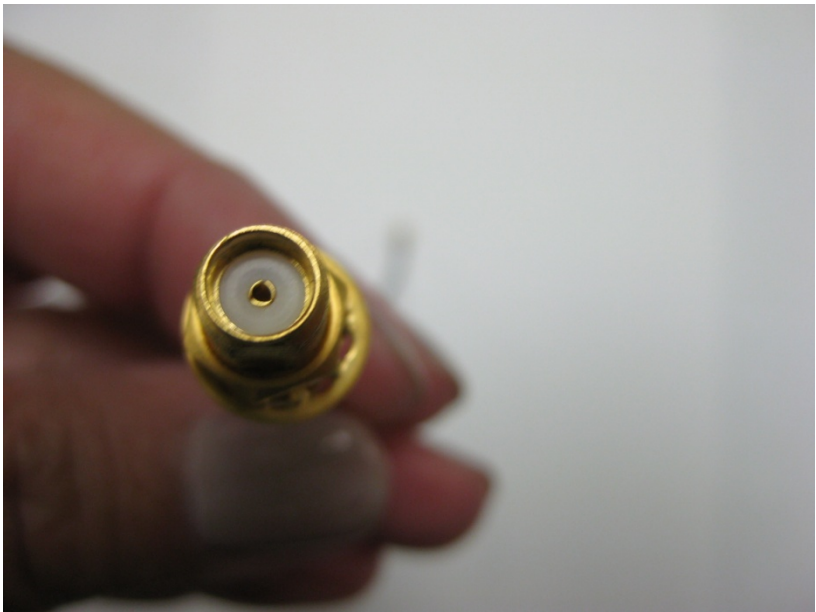
Close Up of U.FL to SMA Cable (Model EM-0069B)
