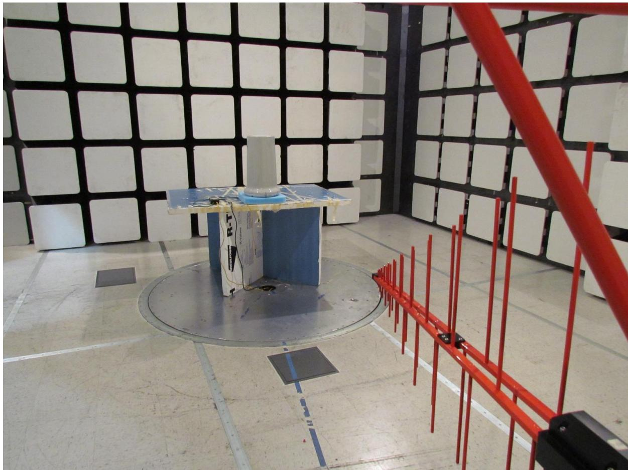
Radiated Emissions Above 1 GHz - Test Setup
