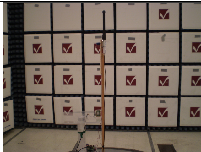
View of 6dBi fixed antenna
