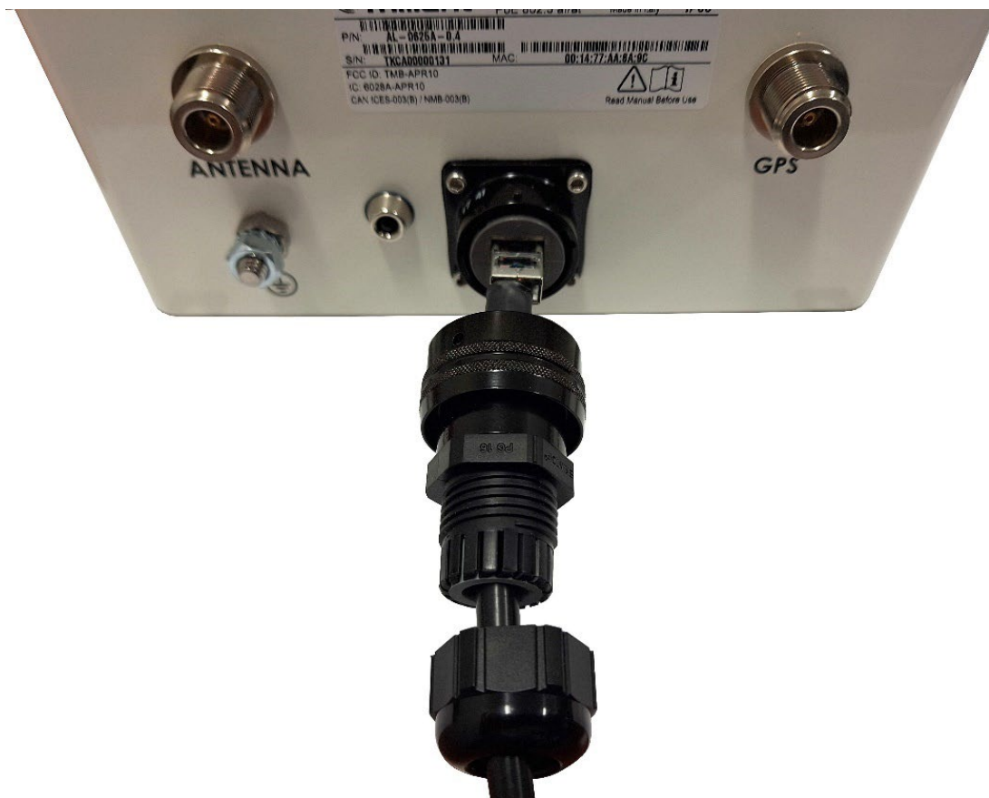
Figure 12: Coax cable through backshell items
