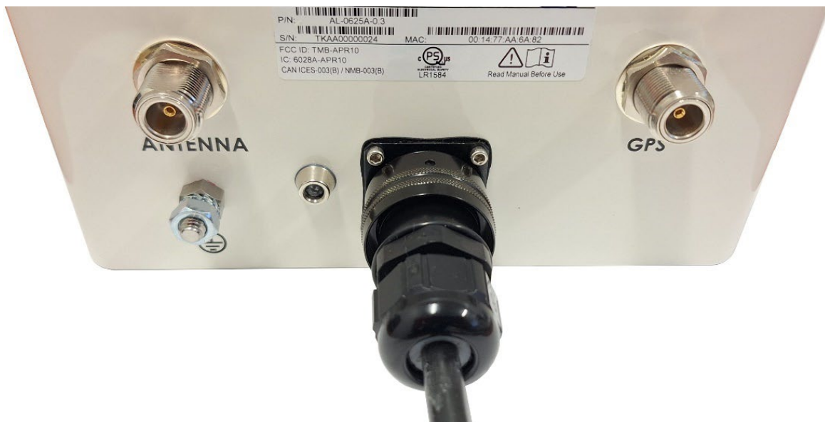
Figure 14: Gland installed and gasket compressed
