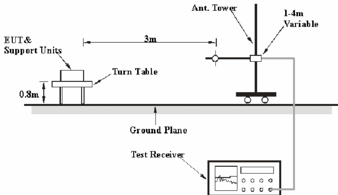
The radiated emission tests were performed in the 3 meters chamber B test site, using the setup accordance with the ANSI C63.4 - 2003. The specification used was the FCC Part 15.209 and FCC Part 15.239.
