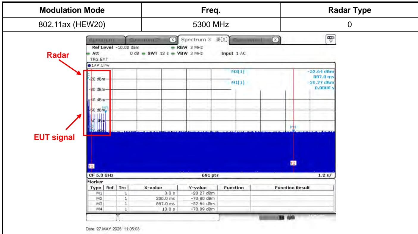
**In-Service Monitoring for Channel Closing Transmission Time (CCTT)**
