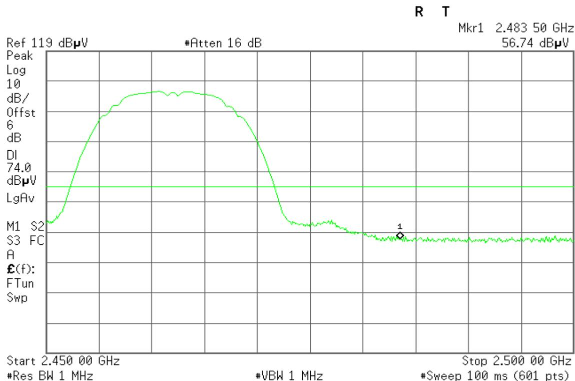
**Detector mode: Average****Polarity: Horizontal**
