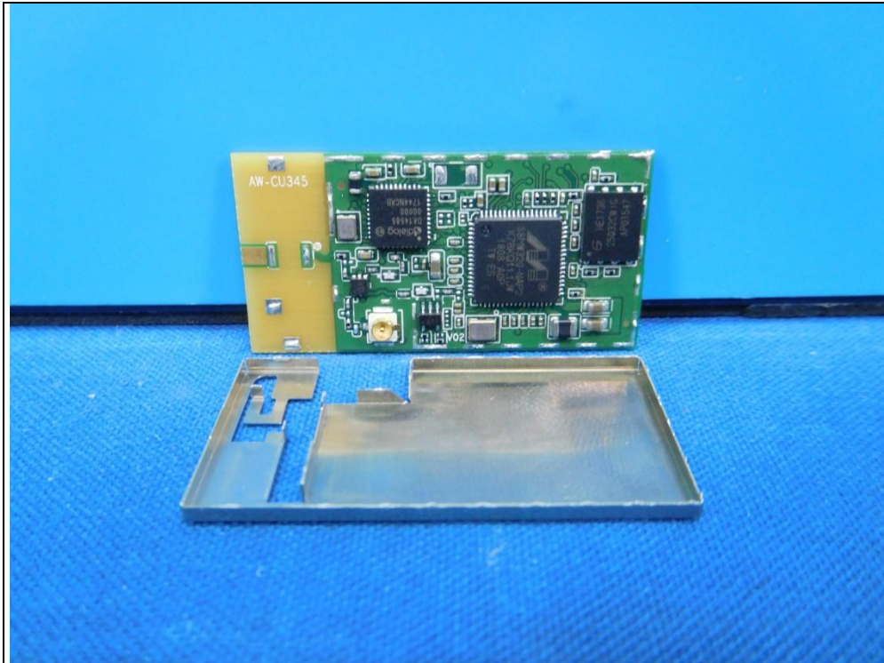
Flash chip No. 2 (Brand: GigaDevice, Model: GD25Q32 series)
