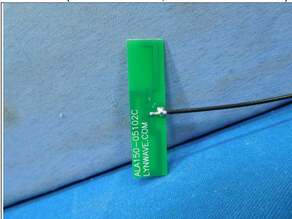
Antenna 31 (Brand: LYNWAVE ; Model: ALA150-05102C)
