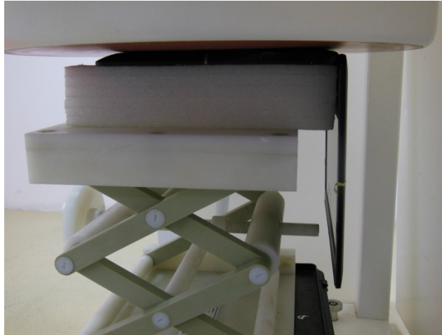
Bottom of Laptop, Test Separation 0 cm
