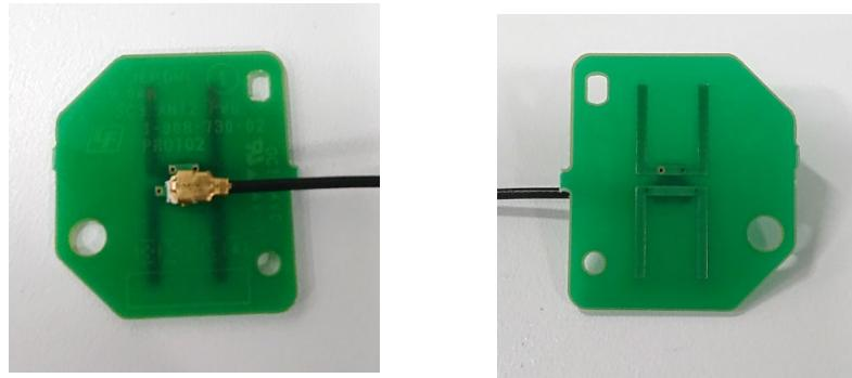
The difference between IW416-D and IW416-G is only substrate material. Antenna pattern is same.
