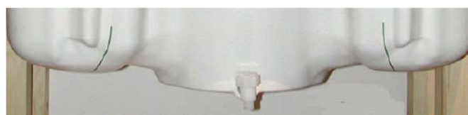
Figure 7.2 SAM Twin Phantom shell
