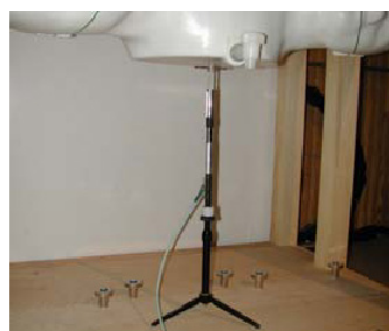
Figure 12.1 Dipole Validation Test Setup
