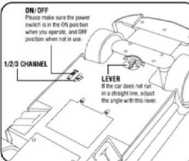
The vehicle has three channels per frequency, please make sure the channel switch is in the corresponding position that is matched to the position of channel switch on the transmitter before operating.
