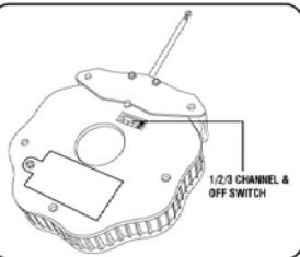
The transmitter has three channels per frequency, please make sure the channel switch is on the corresponding position that is matched to the position of channel switch on the vehicle before operating.
