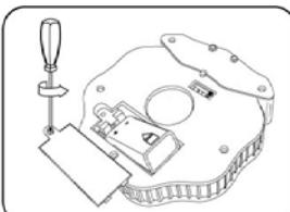
Install one 9V battery with polarity (+/-) as shown inside battery compartment (not included).
