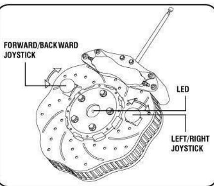
Change the angle of FORWARD/BACKWARD joystick can change the vehicle's speed from slow to fast or from fast to slow.
