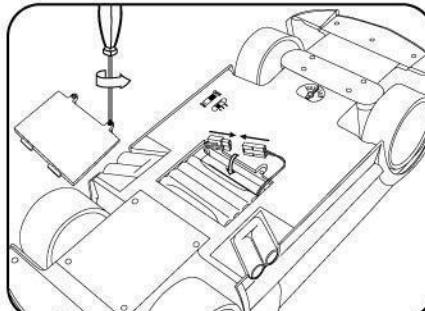
Remove battery door with a Philips head screwdriver (not included) and attach the 9.6V battery pack to the play inside battery compartment with polarity (+/-).
