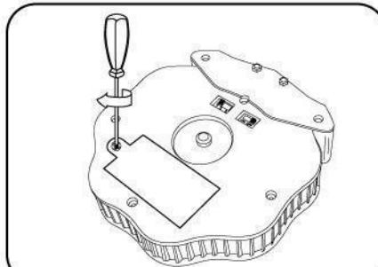
Tighten battery door with a Philips head screwdriver (not included).
