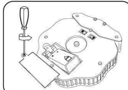
Install one 9V battery with polarity (+/-) as shown inside battery compartment.
