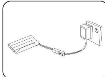
Attach the 9.6V Ni-Cd battery pack to the battery charger, then plug the battery charger into a standard wall outlet.
