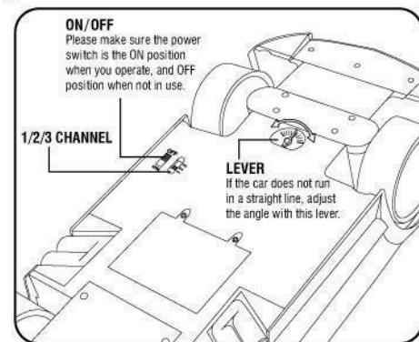
The vehicle has three channels per frequency, please make sure the channel switch is on the corresponding position matched the position of channel switch of the transmitter before play.
