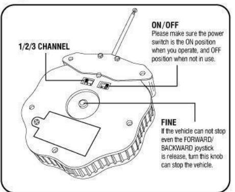
The transmitter has three channels per frequency, please make sure the channel switch is on the corresponding position matched the position of channel switch of the vehicle before play.
