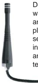
Designed for permanent attachment, PW Series 1/4-wave whips give outstanding performance in a rugged and cost-effective package. The antenna is attached by placing its base through a 1/4" hole in the product and securing it with a nut or by threading it into a PEM-style insert. The antenna attaches to a PCB or connector via an 8½-inch RG-174 coax cable. Custom lengths and terminations are available by special order.
