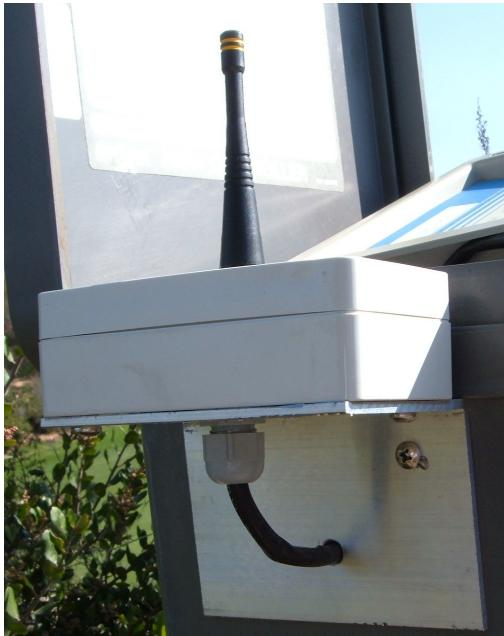
The Pedestal Repeater Configuration unit is designed to be used above ground with the antenna oriented towards the sky. For convenience it can be co-located with irrigation satellite pedestals.
