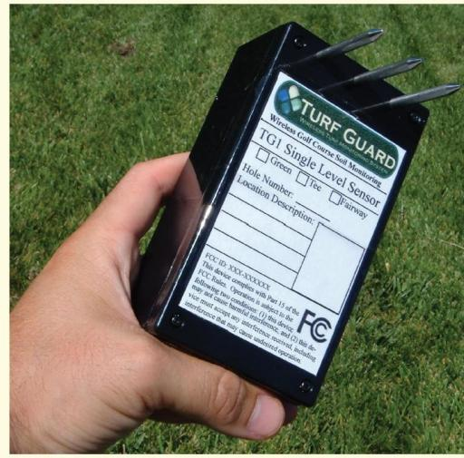
The in ground unit is designed to be fully buried in soil below the turf level. It does not have any user serviceable parts. Do not attempt to open the unit. If the external plastic case becomes damaged in any way, please discontinue use of the device.
