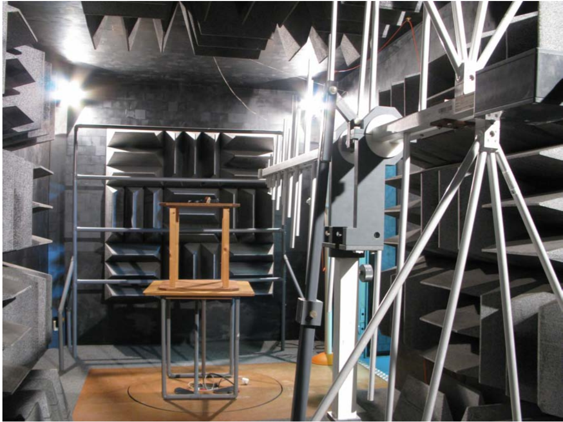
Photograph 9: Test setup exploratory measurements 30 - 1000 MHz
