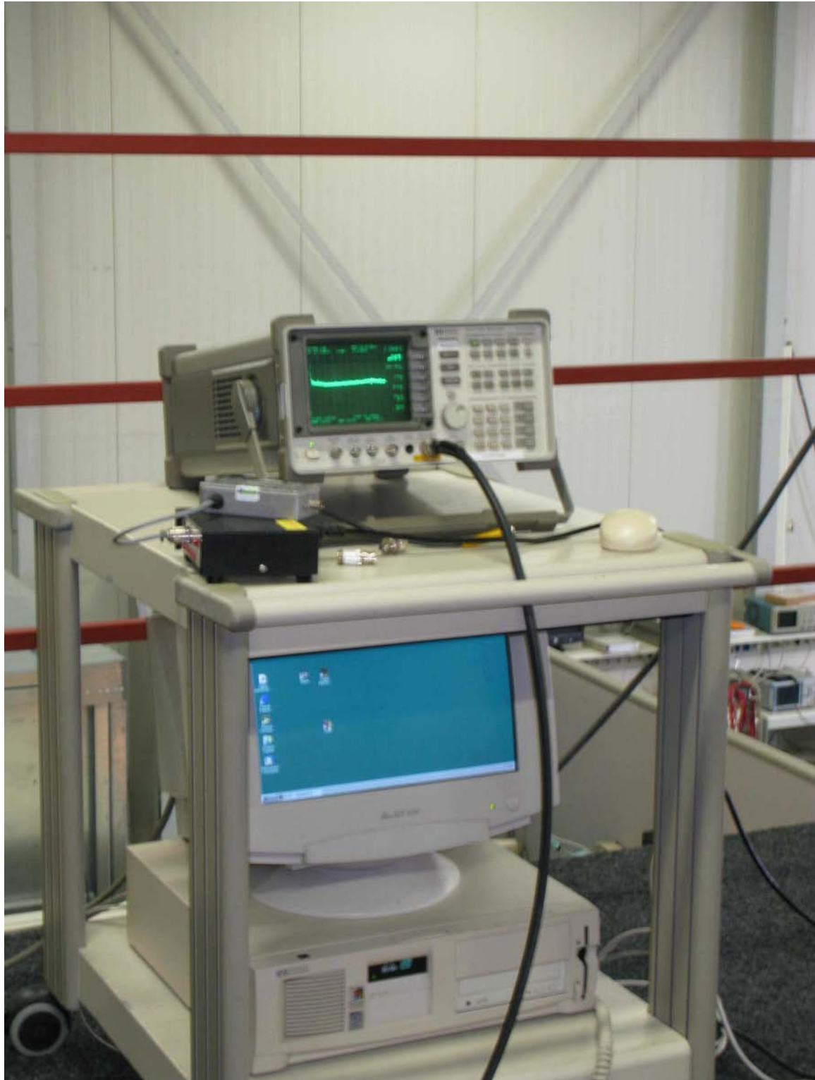
Photograph 2: Test setup exploratory measurements 9 kHz - 30 MHz
