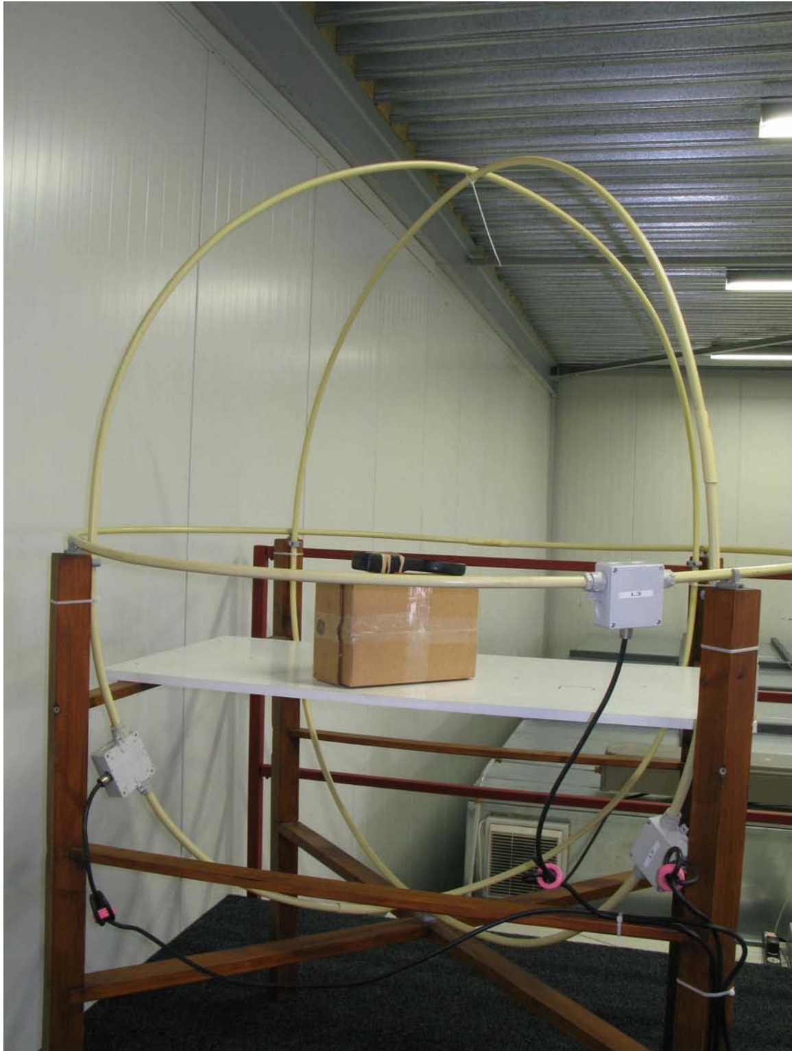
Photograph 1: Test setup exploratory measurements 9 kHz - 30 MHz
