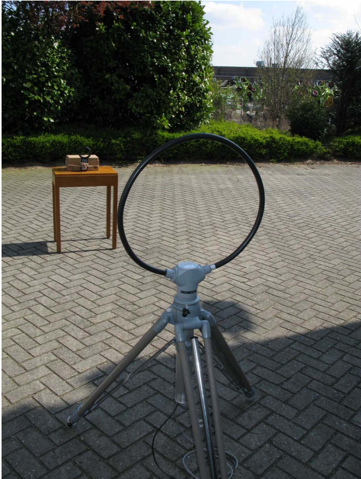
Photograph 6: Test setup compliance measurements 9 kHz - 30 MHz
