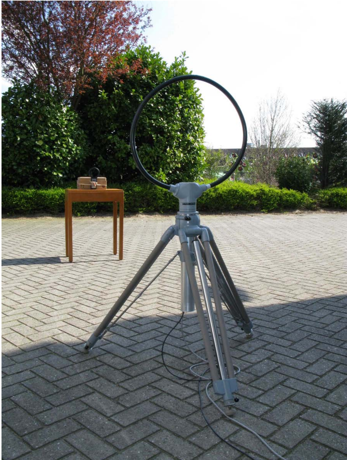
Photograph 5: Test setup compliance measurements 9 kHz - 30 MHz
