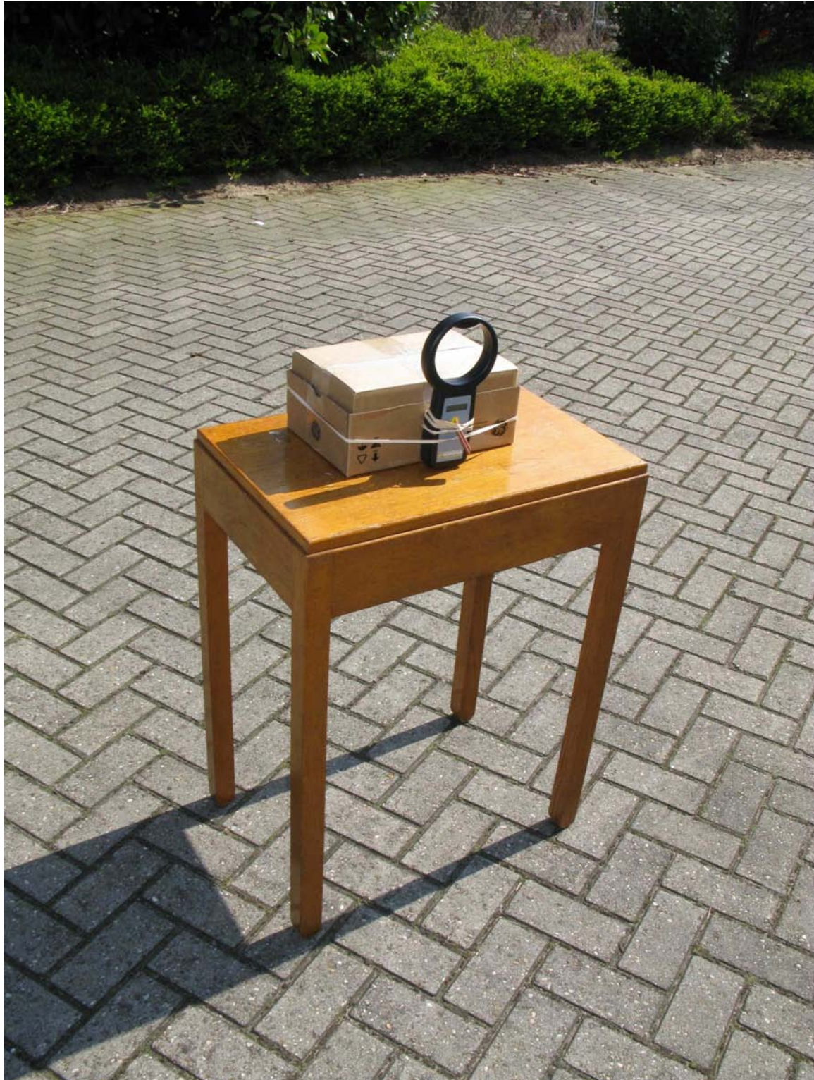
Photograph 3: Test setup compliance measurements 9 kHz - 30 MHz
