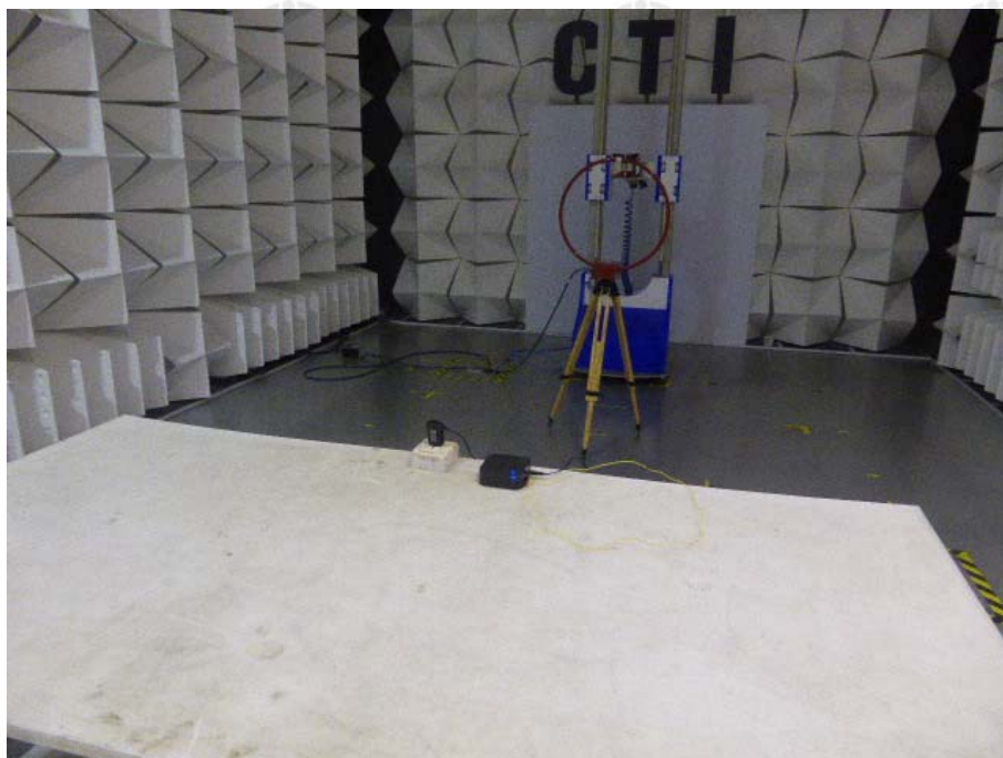
Radiated emission Test Setup-1(9kHz~30MHz)
