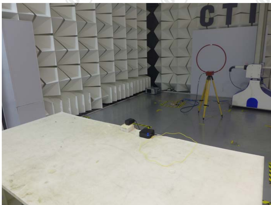
Radiated emission Test Setup-2(9kHz~30MHz)
