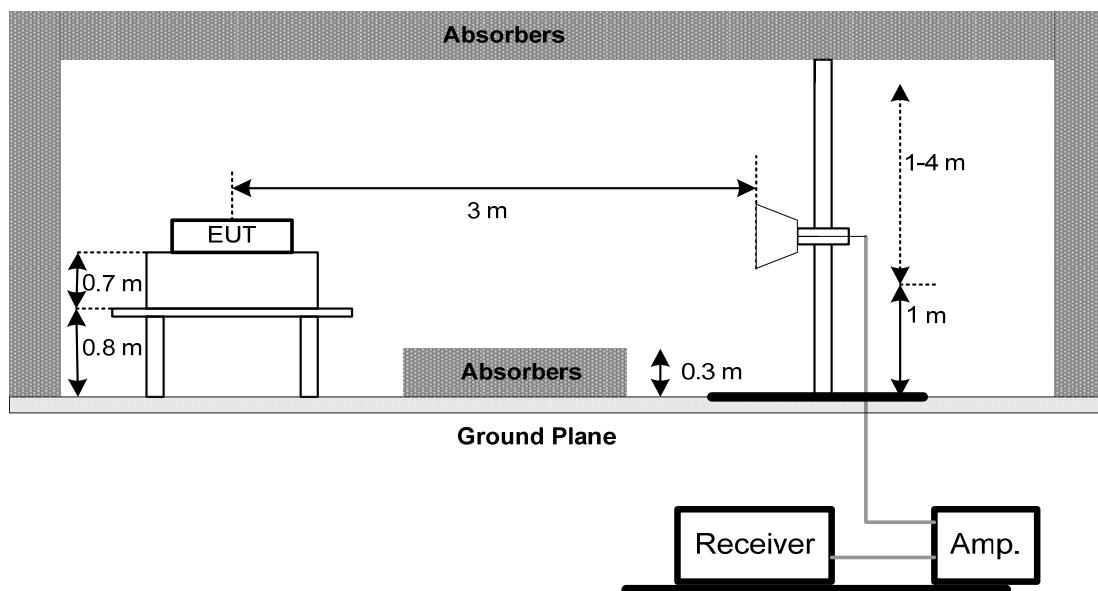
(C) For Radiated Emissions Below 30MHz
