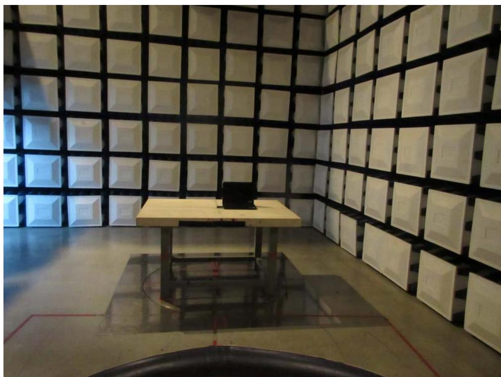
**Radiated Measurement Photos****30MHz to 1000MHz**
