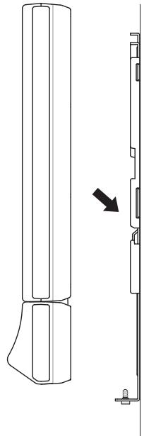
**3** Connect X-Station 2 to the bracket by rotating the product fixing screw of X-Station 2.
