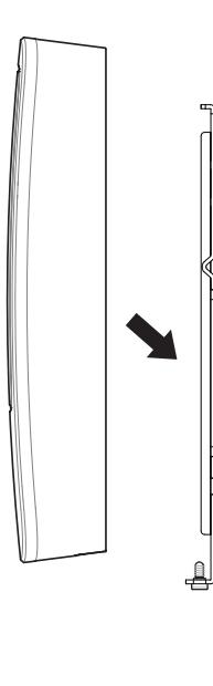
**3** Assemble XPass 2 with the bracket by rotating the product fixing screw.
