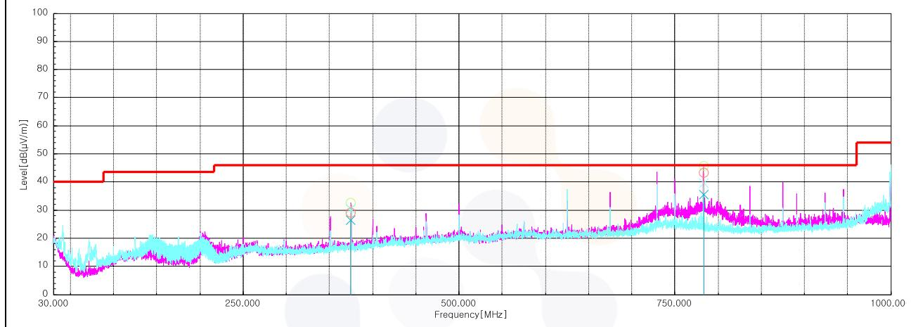
**Test results (Above 1 000 MHz)\_1 MBits/s(37 Bytes)****2 402 MHz**
