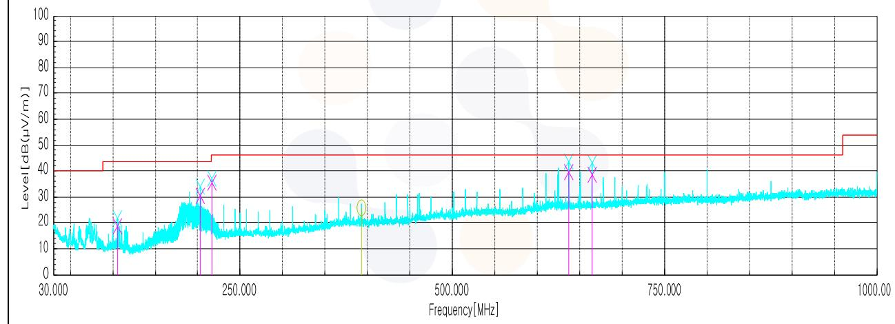
**[PoE]****Test results for fundamental****15.225 (a) 13.553-13.567 MHz****[Face-on]**
