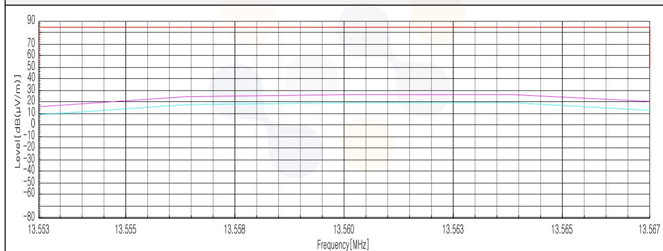
**Test results for in-band & out-band (9 kHz to 30 MHz)****15.225 (b,c) 13.110-14.010 MHz**
