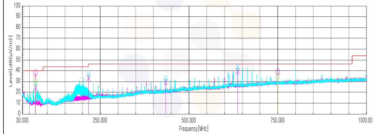
**[DC 24 V]****Test results for fundamental****15.225 (a) 13.553-13.567 MHz**
