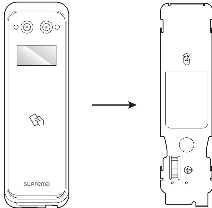
4 Connect BioEntry W3 to the bracket by rotating the product fixing screw of BioEntry W3.
