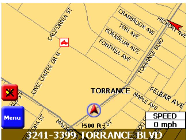
If you do not have a GPS signal, the map defaults to the last location. The vehicle icon displays as a green, yellow, or red arrow on the map. The color indicates the number of available satellites. At the bottom of the map is the vehicle location.
