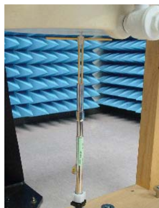
Photograph of the 900MHz dipole Antenna
