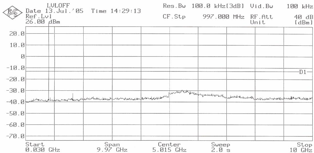
Note: The peak above the limit is the carrier frequency.
