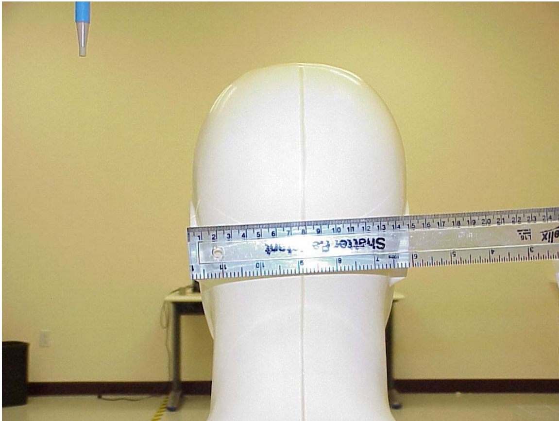
Photo 9. Photo to demonstrate 15 cm Z-axis head phantom
