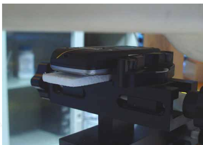
Fig.7 Body worn- EUT back to flat phantom (testing in GPRS Mode and Bluetooth OFF/ON)
