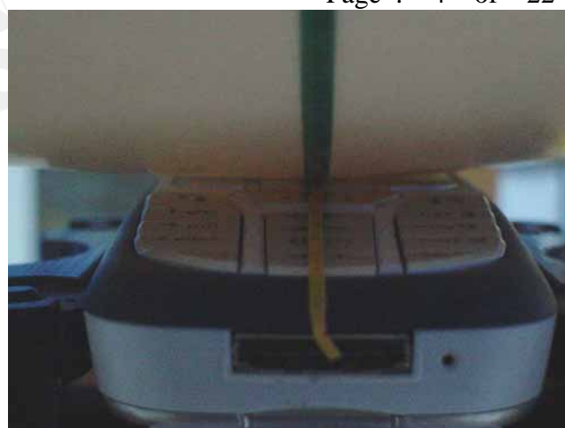
Fig.5 Left Head Section / Cheek-Touch Position
