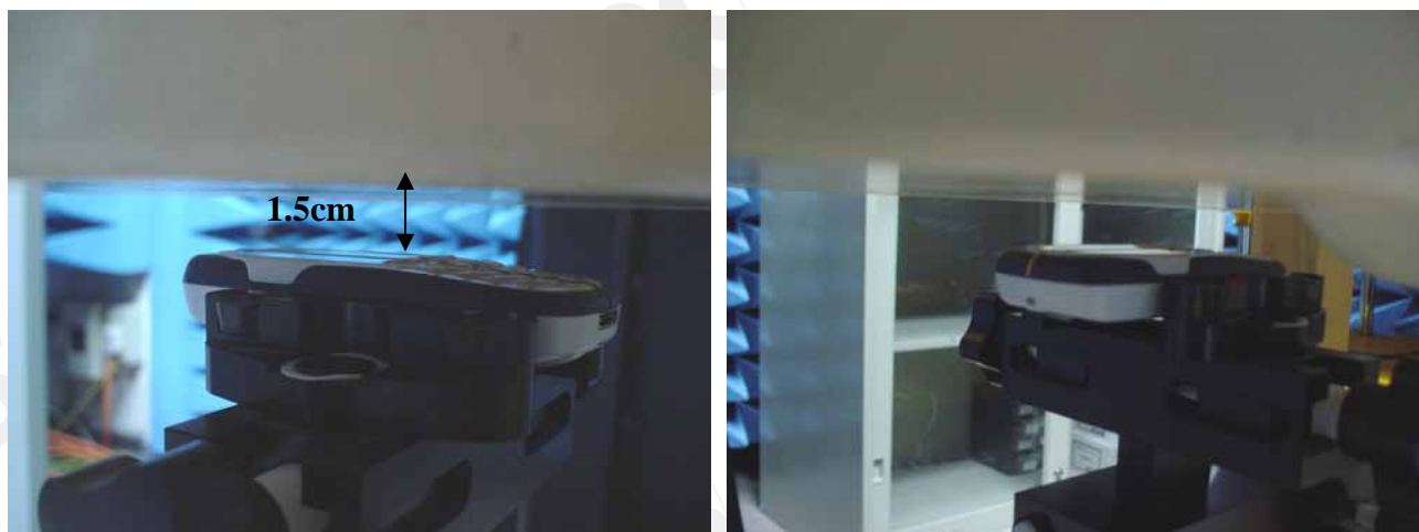
Fig.8 Body worn- EUT front to flat phantom (testing in GPRS Mode)
