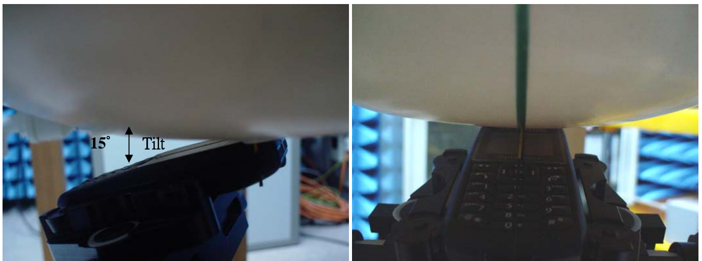
Fig.6 Left Head Section / Ear-Tilt Position(15°)
