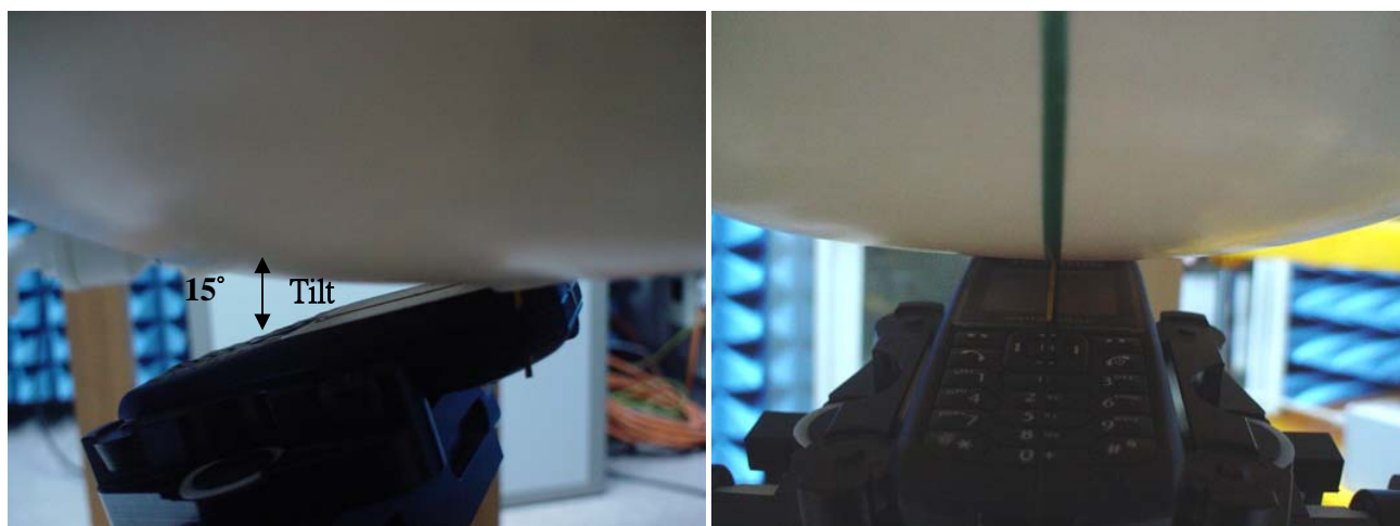
Fig.6 Left Head Section / Ear-Tilt Position(15°)
