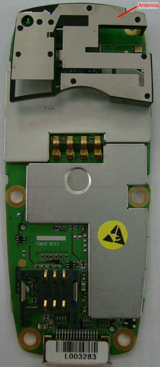
TSM2 PCB with shielding and antenna over it
