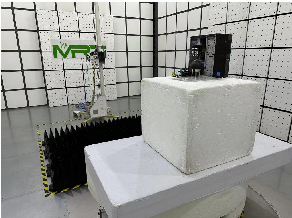
Description: Radiated Restricted Band Edge Test Setup
