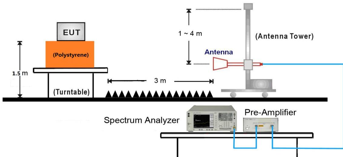
18GHz ~25GHz Test Setup:
