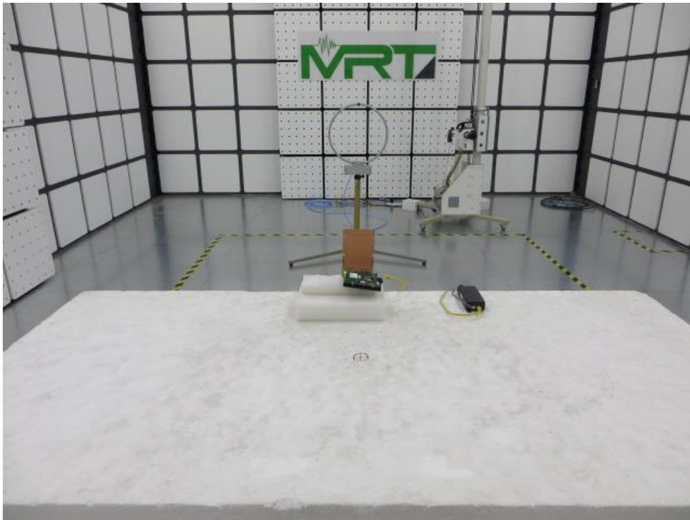
Description: Radiated Emission Test Setup for 30MHz ~ 1GHz (For 2.4GHz Band)
