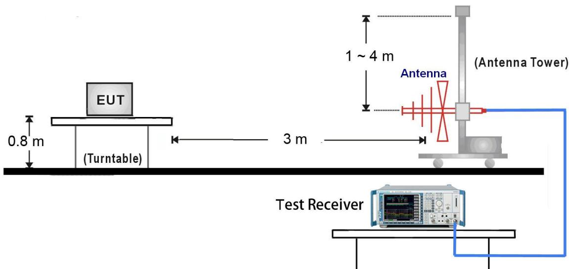
1GHz ~ 18GHz Test Setup:
