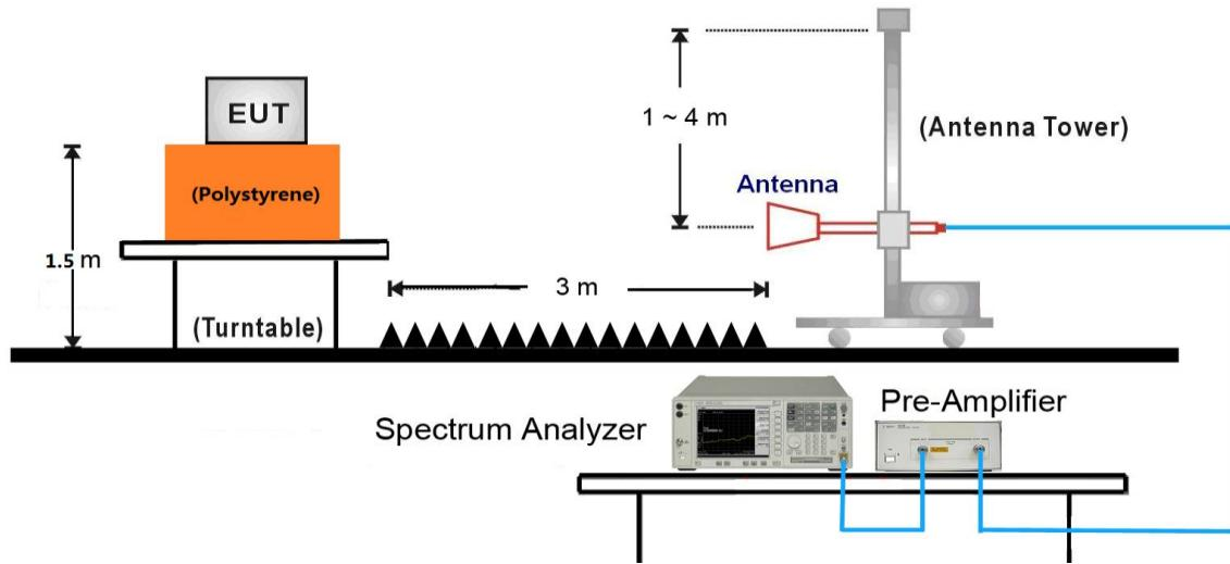
18GHz ~25GHz Test Setup:
