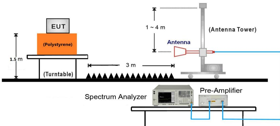
18GHz ~40GHz Test Setup:
